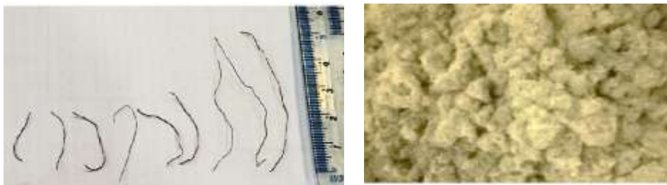
Figure 1. Reused tyre steel fibres (left) and reused tyre polymer fibres (right) after cleaning
