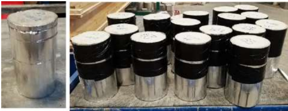
Figure 3. Cutting of cylinders (left) Wrapping of cylinders (right)
